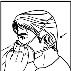
**4** While holding the disposable respirator, bring the top strap over your head and position it around the crown of your head.
