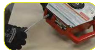
Insert new lifeline into the unit, install shoulder screws and ensure it has engaged.
