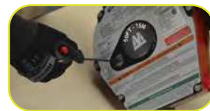
Remove the two shoulder screws on the drum through the side plate cover.
