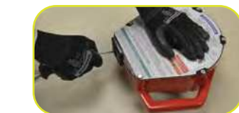
Pull out the entire length of cable until shoulder screws are visible and activate lock.
